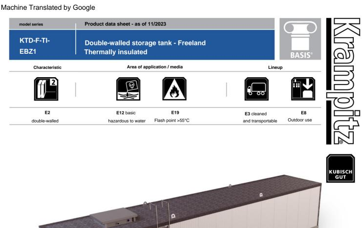
The KTD-F-Ti is used for the storage of mineral oils, lubricating oils, aqueous handheld material solutions or other media that can have problems with pour point and viscosity. Here, the medium is kept flowable by using a tank heater. It is also suitable for... Approved for use in regions with earthquake zone 1. The KTD-F-Ti is manufactured according to the general building regulations approval Z-38.12-312.
