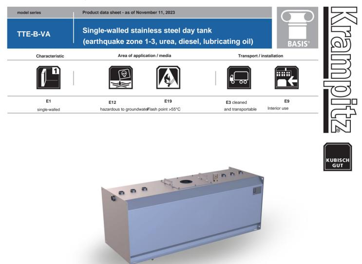
The TTE-B-VA serves as a day tank for supplying units with fuel, urea or lubricating oil. The TTE-B-VA is also known as a storage tank. Due to its structure and features, it meets the requirements for use in emergency power systems in accordance with VDE 107/108. It is suitable for installation in buildings as well as in system containers.
