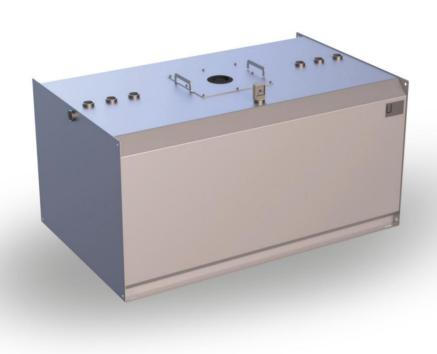
The TTE-C-VA serves as a day tank for supplying units with fuel, urea or lubricating oil. The TTE-C-VA is also known as a storage tank. Due to its structure and features, it meets the requirements for use in emergency power systems in accordance with VDE 107/108. It is suitable for installation in buildings as well as in system containers. The installation surface must be level, load-bearing and designed as a collecting tray. There is none on site
