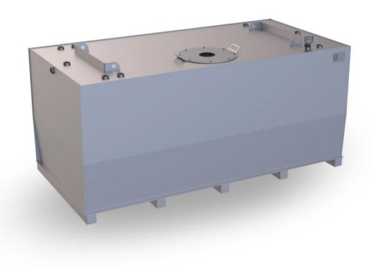
The TTE-XL serves as a day tank for supplying units with fuel or lubricating oil. Due to its structure and equipment, the tank meets the requirements for use in emergency power systems in accordance with VDE 107/108. Due to its volume, the TTE-XL can also function as a storage tank. It is suitable for installation in buildings as well as in system containers. The
